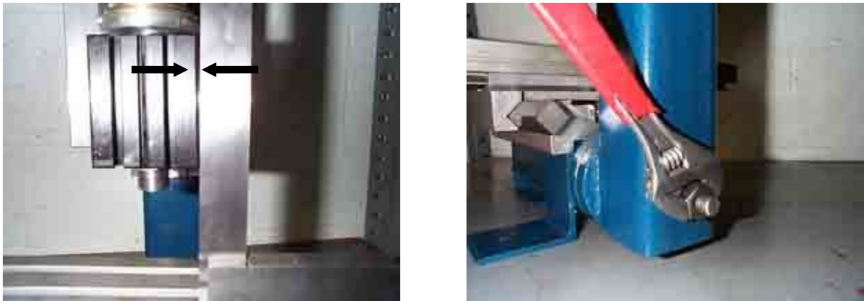
Fig. 4 - Quick squaring of Spindle to Table.
