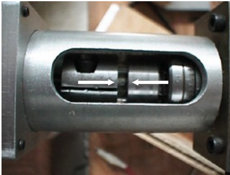
Fig. 3a - Setting the coupling Gap.
