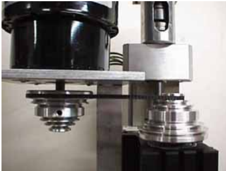
Fig. 9 - Spindle set to top speed position.
