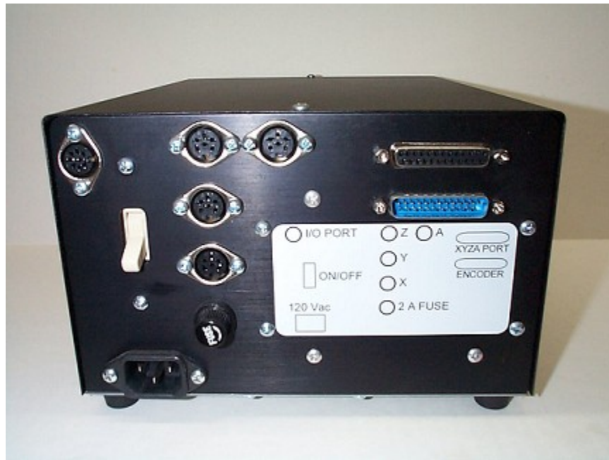
Fig. 3c – Driver box back panel showing axis ports.
