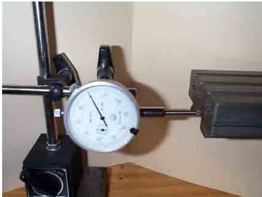
Fig. A3 - Measuring the X-axis Backlash.
